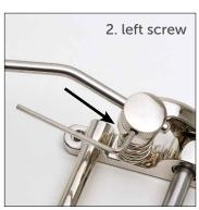
The **mobility of the arm** can be adjusted using the 8 mm locking nut under the arm holder. It is recommended to adjust the nut so that it feels **slightly too tight**.
