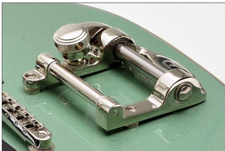
To reduce the angle, the tremolo is „jacked up“. To do this, place washers (e.g. the **Duesenberg Washer Set TDSWSN/TDSWSG**) under the frame of the tremolo at the two front mounting screws. The tremolo's rear edge rests on the top, which ensures a suitable contact angle for the strings.
