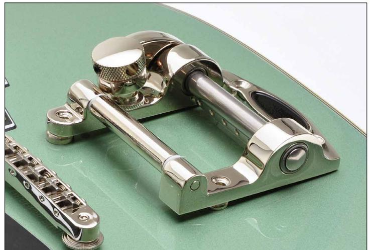
To reduce the angle, the tremolo is „jacked up“. To do this, place washers (e.g. the **göldo Washer Set TGDWSN/TGDWSG**) under the frame of the tremolo at the two front mounting screws. The tremolo's rear edge rests on the top, which ensures a suitable contact angle for the strings.
