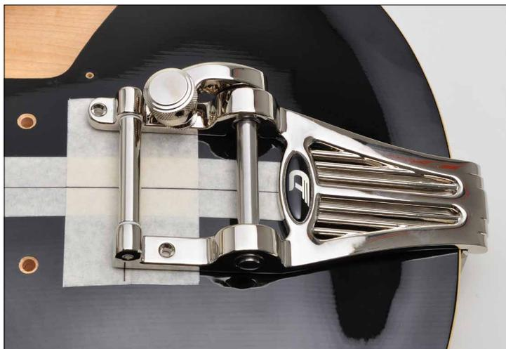
Next, position the two front mounting screws. The lateral position is adjusted by placing a thin thread into the nut and bridge notches of both E strings. The tremolo is then aligned side to side so that the thread has the same distance to both ends of the tension roller. Make sure that the tremolo is perpendicular to the center line. Then mark the positions of the screw holes on the top.
