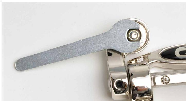
This nut will loosen a little at first. However, it can be readjusted at any time later. To do this, simply lift the arm so that you can remove the spring. The nut can then be adjusted with **the enclosed 8mm wrench**.
